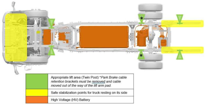
\*Always follow the hoist/lift manufacturers recommendations when operating vehicle lifting devices.
