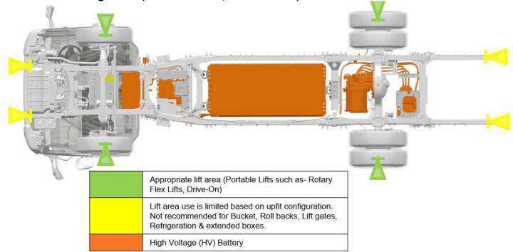
\*Always follow the hoist/lift manufacturers recommendations when operating vehicle lifting devices.
