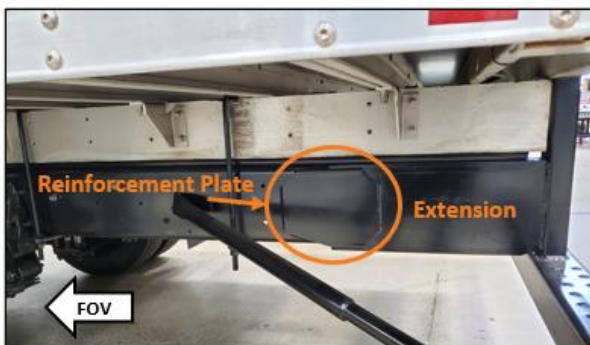
Left frame extension – Outboard View
